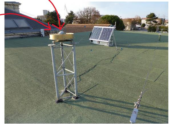
LROC station view from the South. Station has been moved out of the bunker on the 2015/10/16 and is now powered with solar panels and connected through a wifi bridge.
